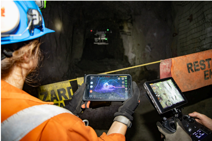
Real-time visualization enables the operator to thoroughly capture a drift and investigate possible problem areas.
