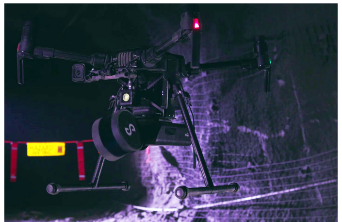
Remote data collection for convergence monitoring helps maintain ground support throughout the mine.
